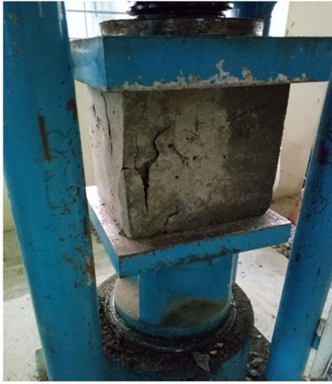
Figure 5: Broken Specimen after Reach Ultimate Load
