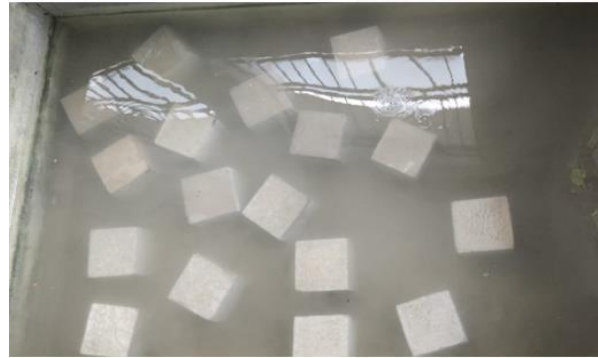
Figure 4: Curing of Concrete Cubes
