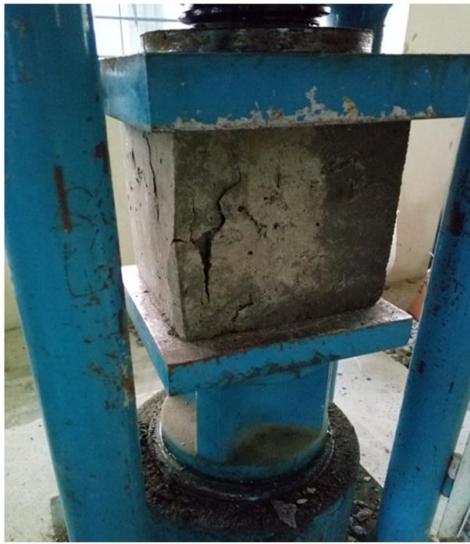
Figure 5: Broken Specimen after Reach Ultimate Load
