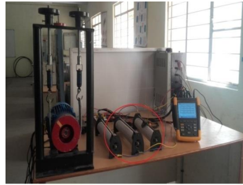
Fig.8. Unbalance voltage is created with help of external resistor
