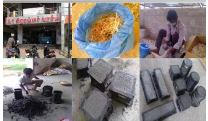
Figure 3: Preparation of Concrete for different Chicken Feather Fibre (CFF) Proportions
